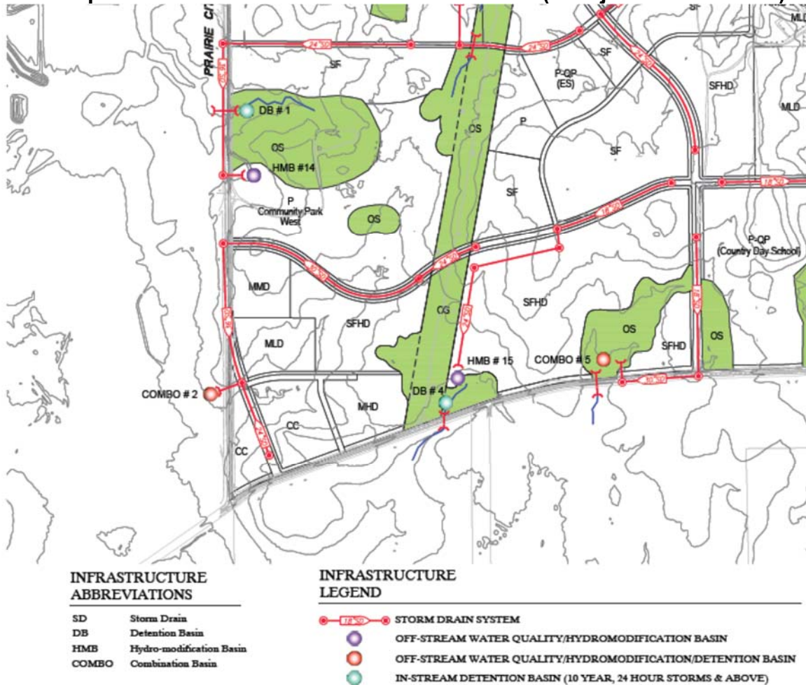
Figure 9 Folsom Plan Area, Storm Drainage Master Plan, Conceptual Backbone Stormwater Infrastructure (Aerojet OU10/Area 40)
